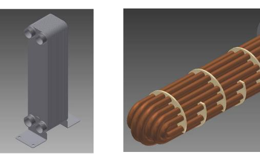
Plate exchangers are ideal for the reasons shown above with lower temperature heating medium and potable water. They are not recommended for use with hard water. U –tube bundles are still preferred when the heating medium is steam or for higher temperature boiler water systems.
