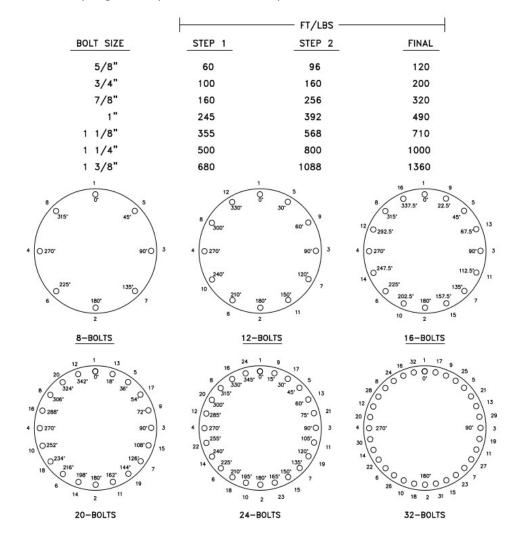
Fig 2.1 - Bolt Tightening Sequence and Torque Values
