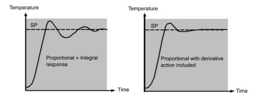
The derivative modifies the output to reduce the rate of change of the difference. It reacts to changes in the PV by changing the output to remove the transient. Increasing the derivative time will reduce the settling time of the loop after a transient change.
