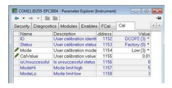
1. Read the DC output on the meter. For a voltage output, this should read 2.00 volts. (For a mA output this should read 4.00mA). If the voltage reading is 1.90V, enter this value, into the C.VAL parameter as shown below.
