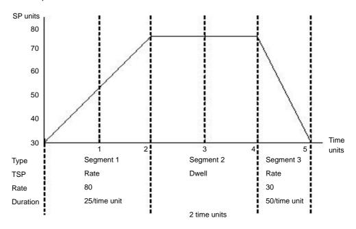
The example above shows a simple three segment program in which the programmer setpoint (PSP) increases at a controlled rate of 25/time unit to a value of 75. It then dwells at that setpoint for 2 time units before decreasing to 30 at a controlled rate of 50/time unit.
