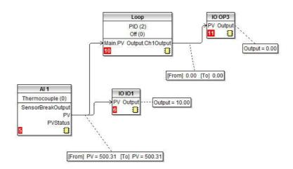
The diagram shows a simple loop where the control output is connected to Output 3 and the PV is wired to Analog Output 1 configured for 0 - 10V.
