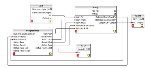
In the figure a thermocouple is connected to Analog Input Al1. The PV output from Al1 provides the input to the control loop. The setpoint for the control loop is provided by the programmer block using the parameter Run.PSP. The programmer will run when the Setup.Run parameter changes to true. In this example the LA digital input may be used to Run/Reset the programmer from an external source.
