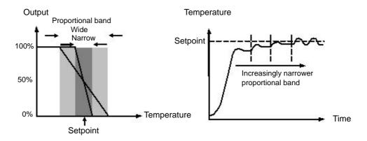
The diagram also shows the effect of narrowing proportional band to the point of oscillation. A wide proportional band results in straight line control but with an appreciable initial error between setpoint and actual temperature. As the band is narrowed the temperature gets closer to setpoint until finally becoming unstable.
