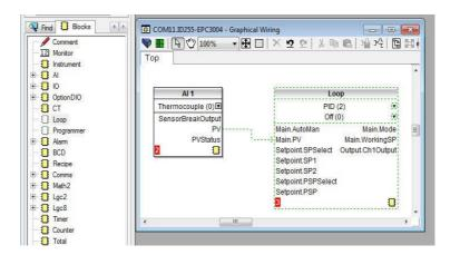
A list of function blocks is shown in the left hand side. Blocks are dragged and dropped from the list into the Graphical Wiring section on the right.
