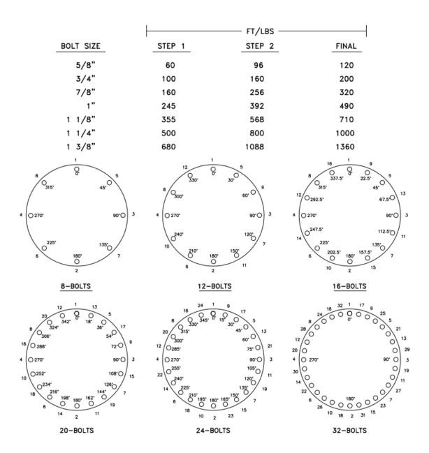
Fig 4.1 - Bolt Tightening Sequence and Torque Values
