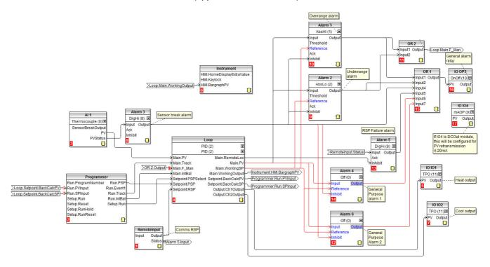
In this example, the sensor input is a thermocouple connected to the main analog input.
