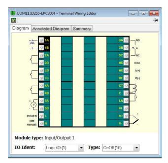
From this view click on a set of terminals representing an IO module. In the 'IO Ident' drop down select an IO type. The diagram of the type of IO will be shown against the chosen terminal set.
